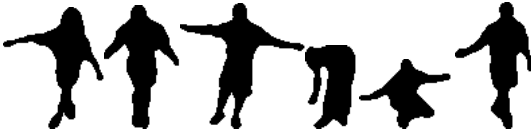
Figure 2: Binary silhouettes of users after figure-ground processing. Task-dependent vision routines to find hands and pose information use this representation as input.
