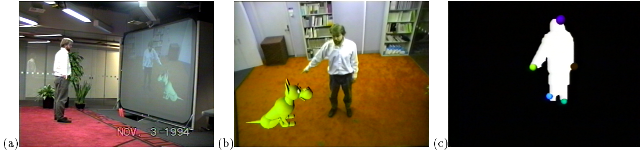
Figure 3: The ALIVE system for vision-based interaction with a virtual environment. (a,b) A user sees him/herself in a “magic mirror”, composited in a virtual environment. Computer vision routines analyze the image of the person to allow him/her to effect the virtual world through direct manipulation and/or gestural commands. (c) Results of hand and head tracking routine. The resolution of hand images from the single camera in previous versions of ALIVE was insufficient to apply the view-based recognition techniques; hand gestures were modeled only using the motion of the hand location. Adapted from [2].
