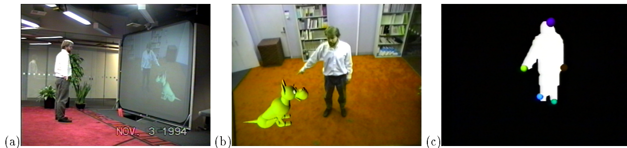
Figure 2: Person tracking in a system for vision-based interaction with a virtual environment. (a,b) A user sees him/herself in a “magic mirror”, composited in a virtual environment. Computer vision routines analyze the image of the person to allow him/her to effect the virtual world through direct manipulation and/or gestural commands. (c) Results of feature tracking routine; head, hands, and feet are marked with color-coded balls.
