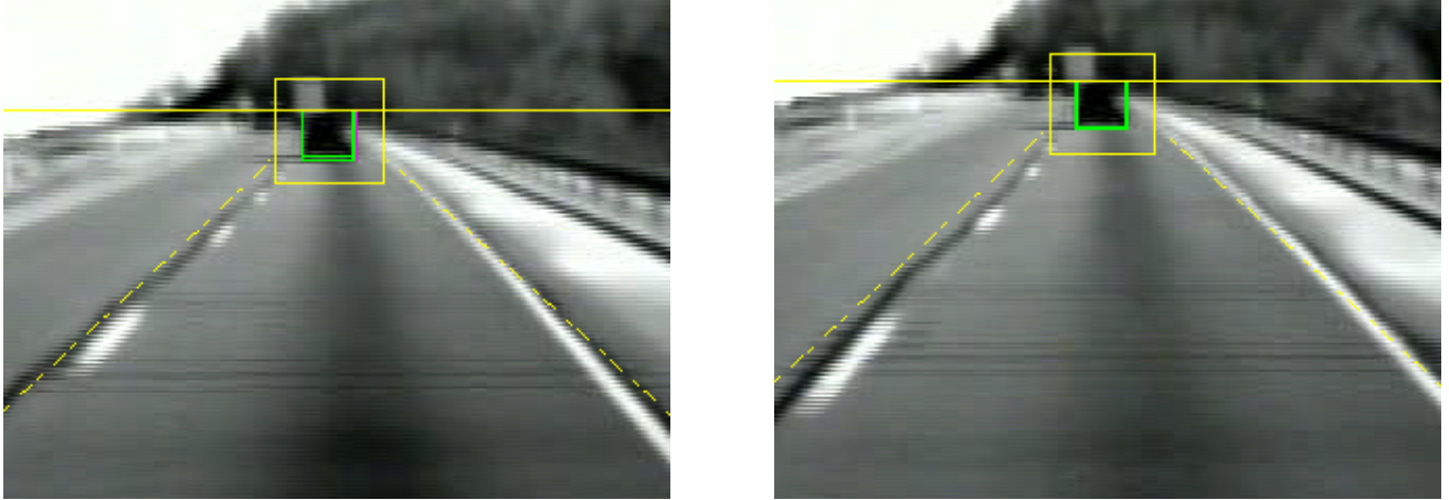
Figure 7. Image stabilization. Two frames (one close after the other around t = 750 ) illustrating image stabilization by augmenting the state vector with pitch, modeled as colored (time correlated) noise.
