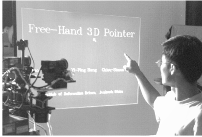
Figure 2. This figure illustrates the operation of our free-hand pointer. The speaker is pointing his index finger to the projection screen (under the word “3D”). The IIS head on the left takes the stereo image pairs to be processed. According to the projection site determined from the stereo image pairs, the computer then controls its cursor to the word “3D”.
